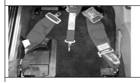
Picture of how the aftermarket lap belts Look with the seat removed. Torque all bolts
