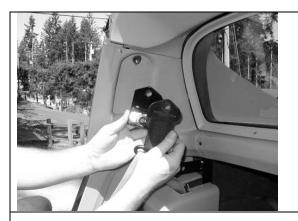
1. Re-Install the *factory 1/2" sail harness shoulder bolt* through the shoulder harness guide, sail bracket and the shoulder harness guide cover into the sail anchor bolt hole.
