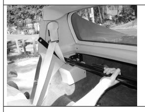
3. Carefully maneuver the harness bar into place with the OEM shoulder belts inside of the harness bar struts and in front of the bar.
