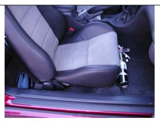
3. Install the Stanguisher extinguisher bracket and install the seat mount nuts and tighten. Place the Amerex bracket onto the Stanguisher bracket using the 3-1/4" button head Allen bolts. Position Amerex fire extinguisher in place and secure straps.
