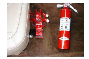
Place the Amerex bracket over the Vetteworks bracket and install the 3 button Allen bolt with a 5/32" Allen wrench.
